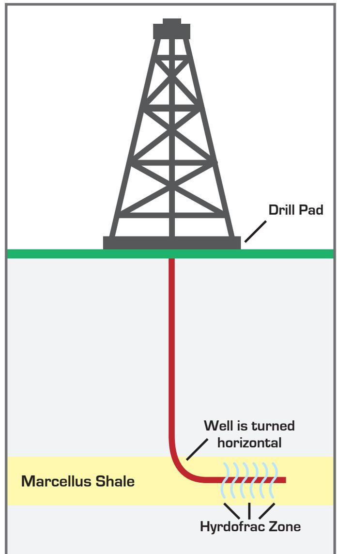
Illustration of a horizontal drill structure. The production ratio for horizontal wells versus vertical wells is 3.2 to 1, while the cost ratio of horizontal versus vertical wells is only 2 to 1.
